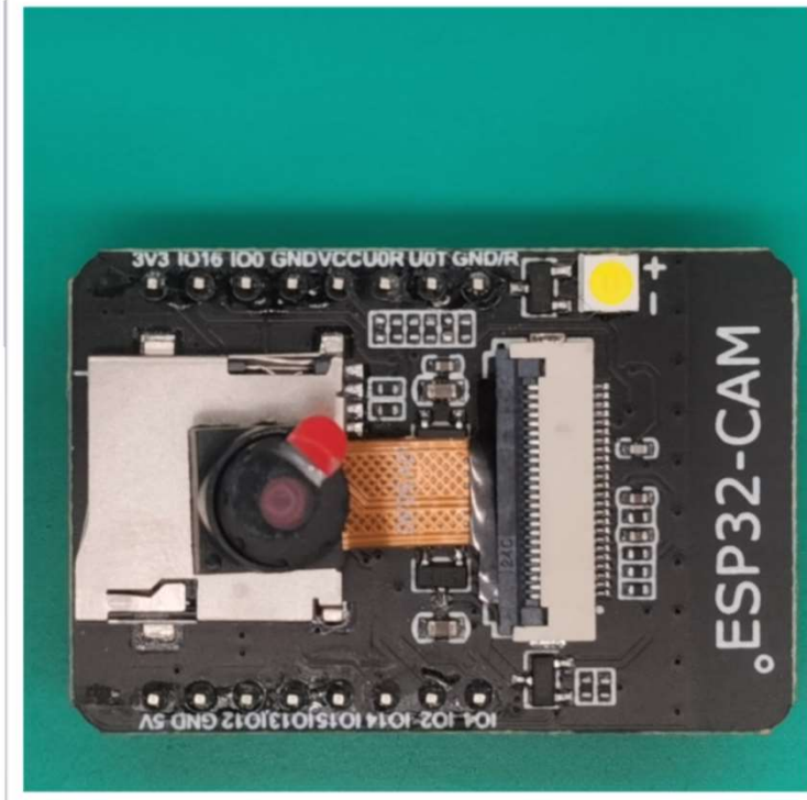
FPC Connector on Camera
